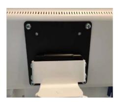
To attach the LCD to the stand. A Phillips Head screwdriver or, if added security is needed for the LCD, a Torx Head driver is needed to attached the LCD to the VESA Stand. Both Phillips and Torx screws are provided. It is recommended that one person hold the LCD while a 2nd person inserts the hardware. Make sure all 4 screws are installed and tightened properly.
