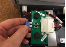
Remove the fuse and review for possible break. You will be able to see if the internal connection is still in place or if it has disconnected. If you have a dual battery system, check both fuses.
