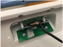
If not seated correctly, position and reconnect. If the front status is still not working, check the other end of the cable connection as shown below. You may need to remove the internal PC to get access to the power inverter. Follow the cable from the front status enclosure and make sure that it is seated properly. Disconnect and reconnect if needed.
