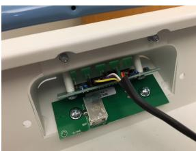
If not seated correctly, position and reconnect. If the front status is still not working, check the other end of the cable connection. Follow the cable from the front status enclosure and make sure that it is seated properly. Disconnect and reconnect if needed.
