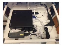
**2. Turn on power to the AC Outlets** – Push the AC Switch shown as item 2 on page 14, to the ON position. This switch can be accessed by opening the rear enclosure door, a blade screwdriver will be needed. The power switch is located on the left side of the inverter/charger assembly as shown below.
